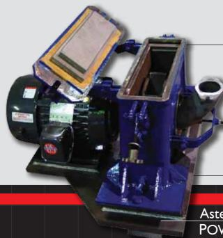
Shot Blast Wheels are mounted in a sealed housing. The inner walls of the wheel housing are subject to extreme abrasive wear caused by shot action. ASTECH manufactures premium wheel housing liners designed to protect housing walls. Our liners are cast with Astech's special chrom-moly white iron alloy. This special alloy is backed by ASTECH'S years of industrial experience in manufacturing long lasting wear components.
